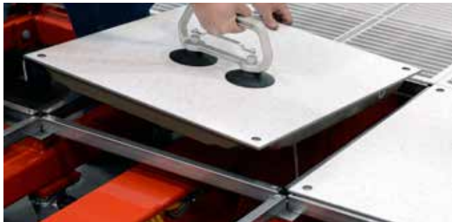
The platforms use standard size computer floor tiles.
