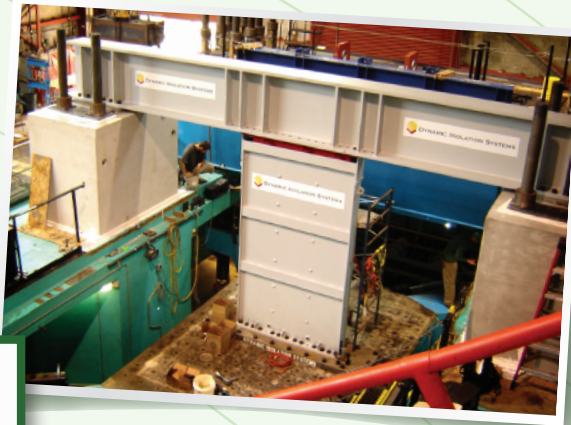
VWD shake table testing at UCSD.
