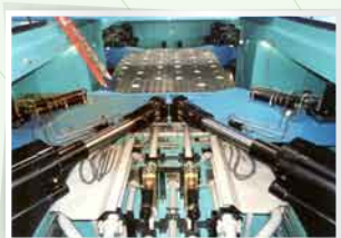
Bearings for the Coronado Bay Bridge were the first to be tested at earthquake velocities at UCSD for Caltrans.
